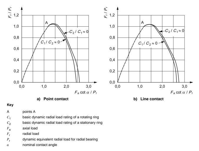
Figure 1 — Dynamic equivalent radial load,  $P_r$ , for single row radial bearings with constant contact angle,  $\alpha$
